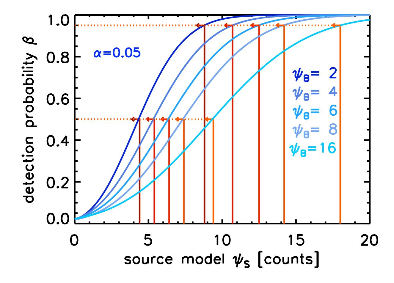
Upper limits for different choices of  $\alpha$ ,  $\mathbf{S}^*$ , and  $\beta_{min}$ , for a background of 5 counts in 10x source area. Curves are for  $\mathbf{S}^*=5, \alpha=0.1$  (solid),  $\mathbf{S}^*=6, \alpha=0.05$  (dashed),  $\mathbf{S}^*=8, \alpha=0.01$  (dash-dotted). Intercepts are for  $\beta_{min}=0.5$  (top), 0.9 (middle), 0.95 (bottom).
